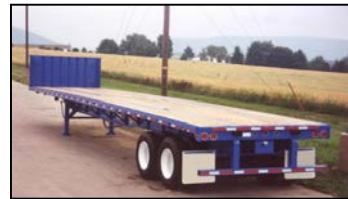
48' or 53' Standard Flatbed aka Drop-Deck, with various configurations of tarps and/or chains
