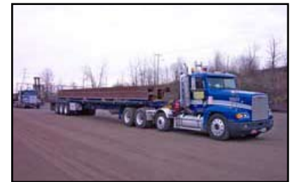
48' or 53' Standard Flatbed aka Drop-Deck, with various configurations of tarps or chains
